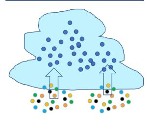
Cloud dissipates leaving behind processed aerosol – some larger and chemically changed.
